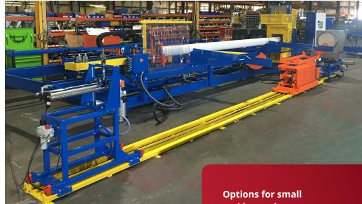
PEM 612 Beller outfited with a hydraulicpowered lift and rotator. PEM lift and rotators are available as stand-alone units or can be integrated into other PEM machinery.
